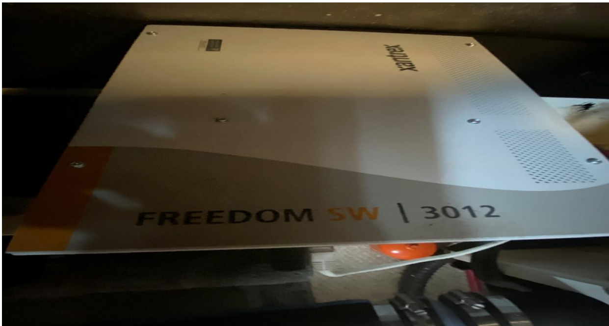
Xantrex - Inverter SW Charger 12VDC-3000W – Generator Support Mode (AC exceeds generator capacity)
